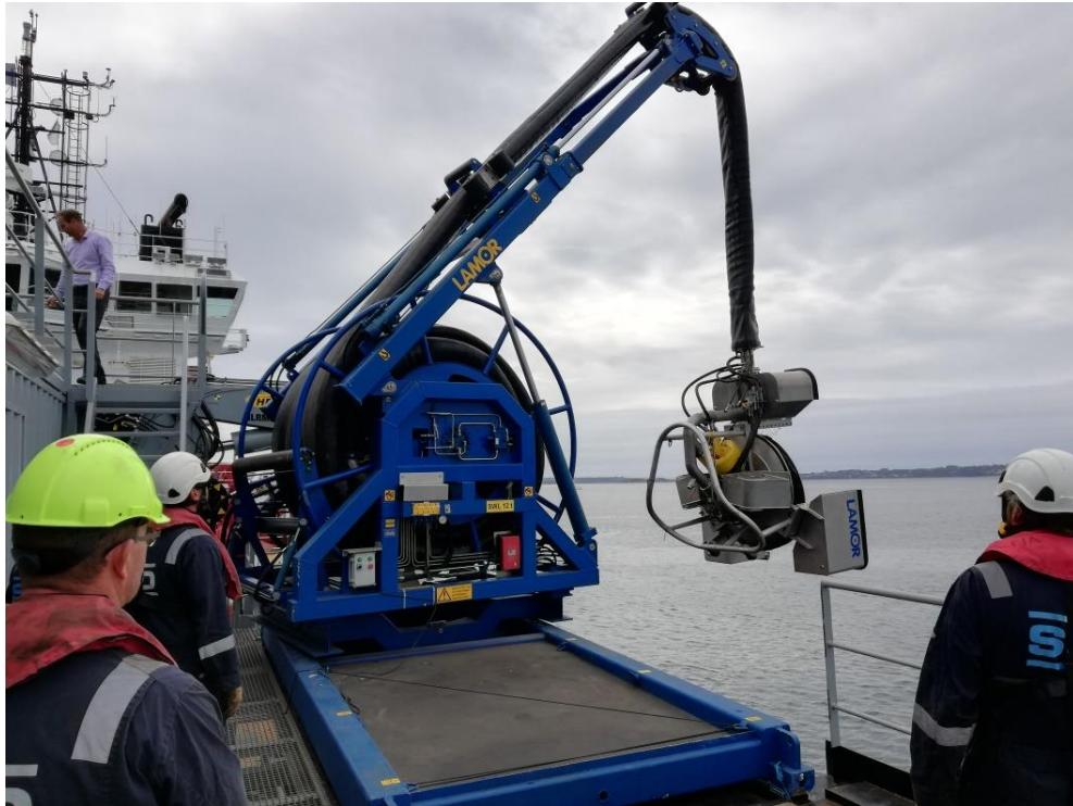
Fig. 15. Umbilical Hose Reel LUT 90, with Telescopic Crane Arm
