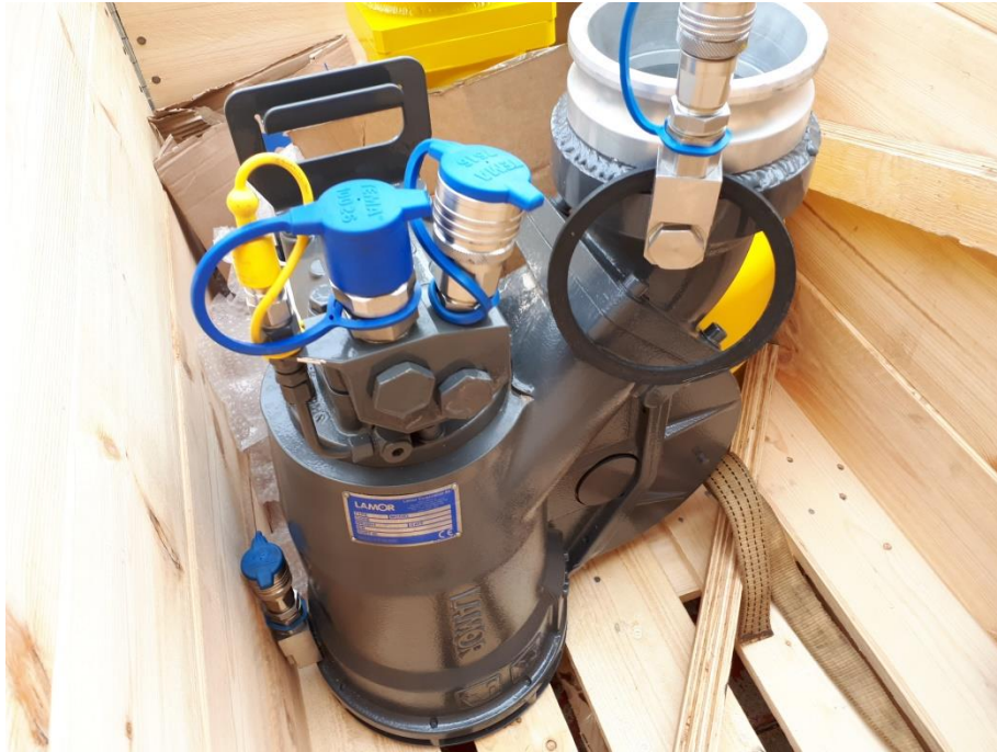
Fig. 21. Oil Transfer Pump GT A 140 PDAS
