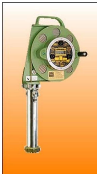
Fig. 26. Oil water interface detector MMC D-2401-2
