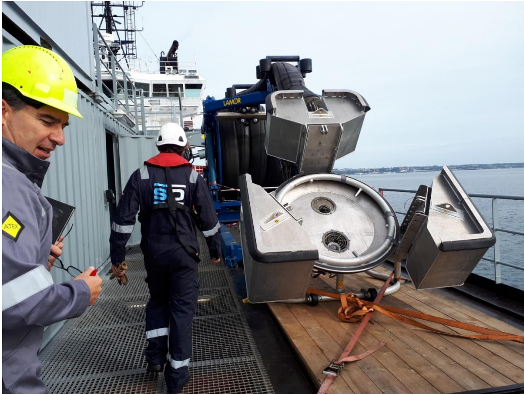
Fig. 19. Lamor Free Floating High Capacity Offshore Skimmer Brush module
