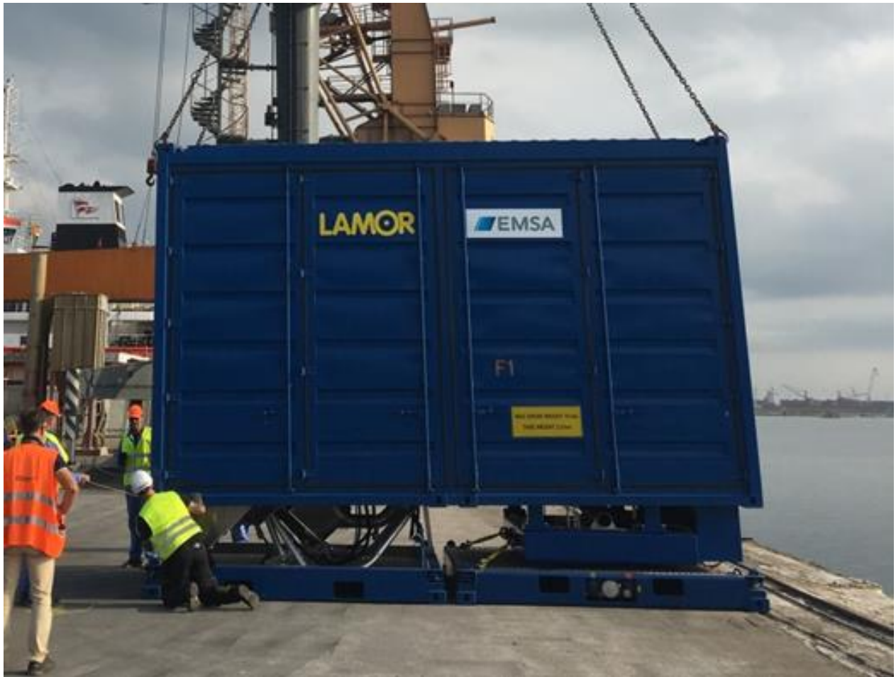
Fig. 22. 20' roof module and 10' bases for skimmer and LUT
