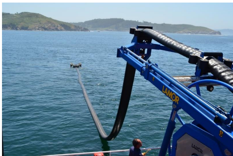
Fig. 16. Umbilical Hose LUH 52 80m, 11 Ch anti-static
