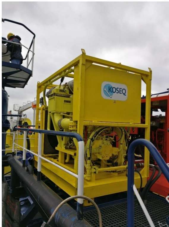
Fig. 8. Diesel-hydraulic power pack for sweeping arms
